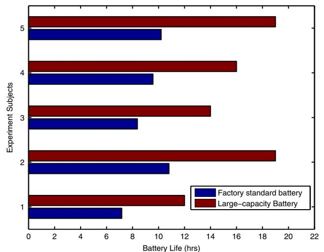
**Fig. 5** The spread of battery lifetime for the original BeWell system. For each person we show battery life using a large capacity battery (3200 mAh) and an estimate of battery life with a standard factory battery (1400 mAh)
