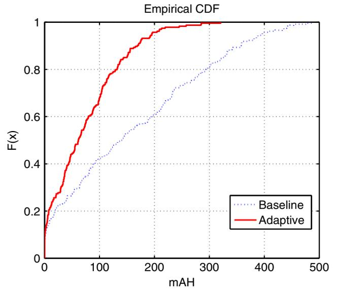
**Fig. 11** CDF of per user daily energy consumption under wellbeing adaptive energy allocation compared to a hand-tuned baseline
